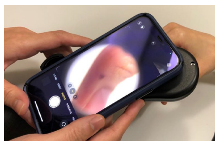
Current prototype of the attachable dermoscope, allowing dermoscopic pictures to be taken via hand phone
